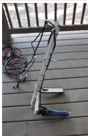
Transducers Blue unit is normal down scan, 2d, and side scan. Other unit is side scan and 3D.
