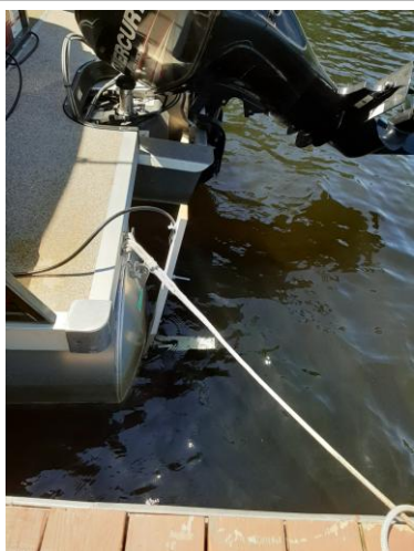
Transducer mounted on pontoon boat
