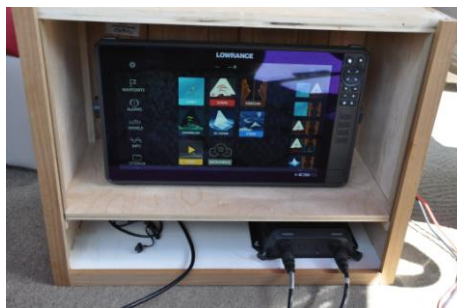
Sonar unit showing display and 3D module
