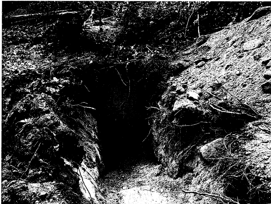
Photograph No. 6: Looking at Test Pit 6B, showing Montauk, very stony soil.
